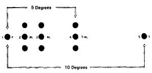
Figure 1. Arrangement of LEDs used to generate visual displays. LEDs 1-5 are numbered on the left. The letters to the right of LEDs 1-5 indicate the function of that LED. F= fixation light, AL= array light, T= target light.
